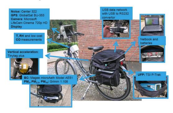
Figure 1. The Aeroflex and its measurement devices.
