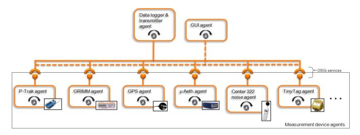
Figure 2. Aeroflex adaptable software architecture with autonomously operating software agents.
