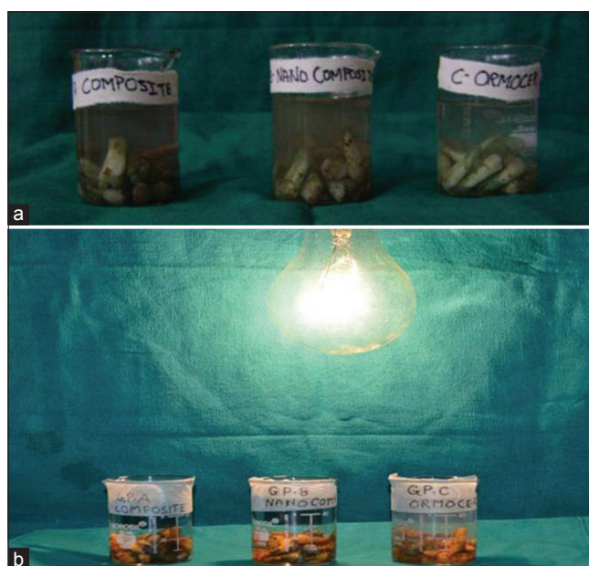
Figure 2: (a) Samples in silver nitrate dye and (b) samples in developing solution
