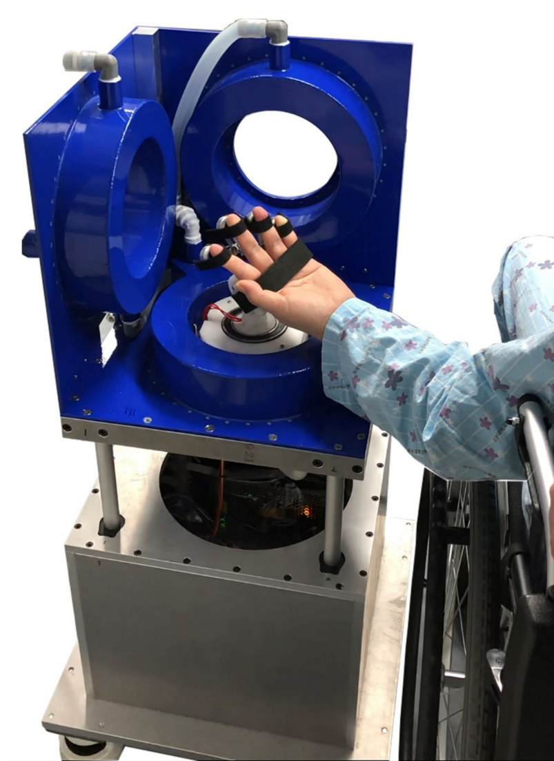
Figure 1. 3D magnetic-force-driven finger rehabilitation device. The installed magnet-array device on the patient's fingers generates magnetic attractive and repulsive forces by the driving magnetic field in the 3D coil system. Rehabilitation therapy can be performed by assisting the movement of the paralyzed fingers using these magnetic forces.
