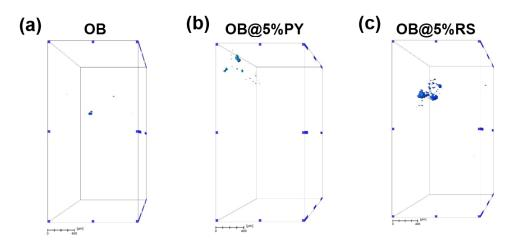
**Figure 9.** Micro-computed X-ray tomography analysis (scale bar of 400  $\mu$ m). Volume rendering of the segmented pores in (**a**) OB (unmodified sealer); (**b**) OB@5%PY (sealer doped with 5%PY); and (**c**) OB@5%RS (sealer doped with 5%RS).
