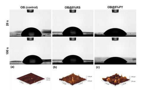
**Figure 7.** Contact angles of a water droplet (initial volume of 8  $\mu$ L) deposited onto different composite surfaces (OB, OB@5%RS and OB@5%PY) after 20 and 100 s post deposition. AFM micrographs (20  $\mu$ m × 20  $\mu$ m) of the different composite surfaces (**a**) OB, (**b**) OB@5%RS and (**c**) OB@5%PY.
