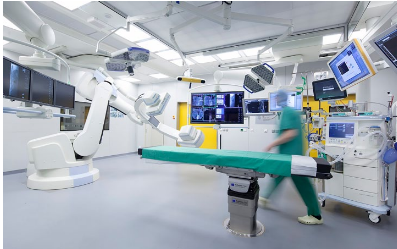
Fig. 2 Hybrid operating room - floor-based 3D flat-panel detector with cone-beam CT capability and fully integrated navigation system.
