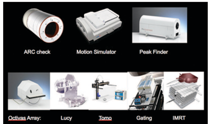
Figure 13: Radiotherapy dosimetry QA phantoms — top row: ArcCHECK, motion simulator, peak finder; bottom row: Octavis array, Lucy, Tomo, gating and IMRT
