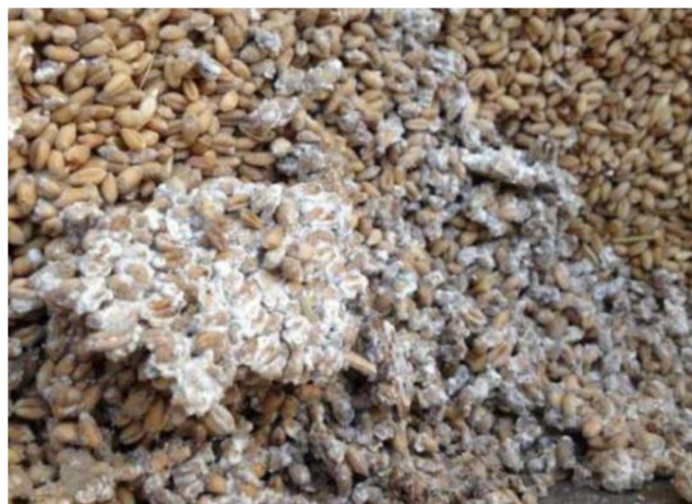
Figure 5. Spoiled (mouldy) grain found at location B (0.8 m from the bin bottom and 0.4 m from the cold wall) on day 60.
