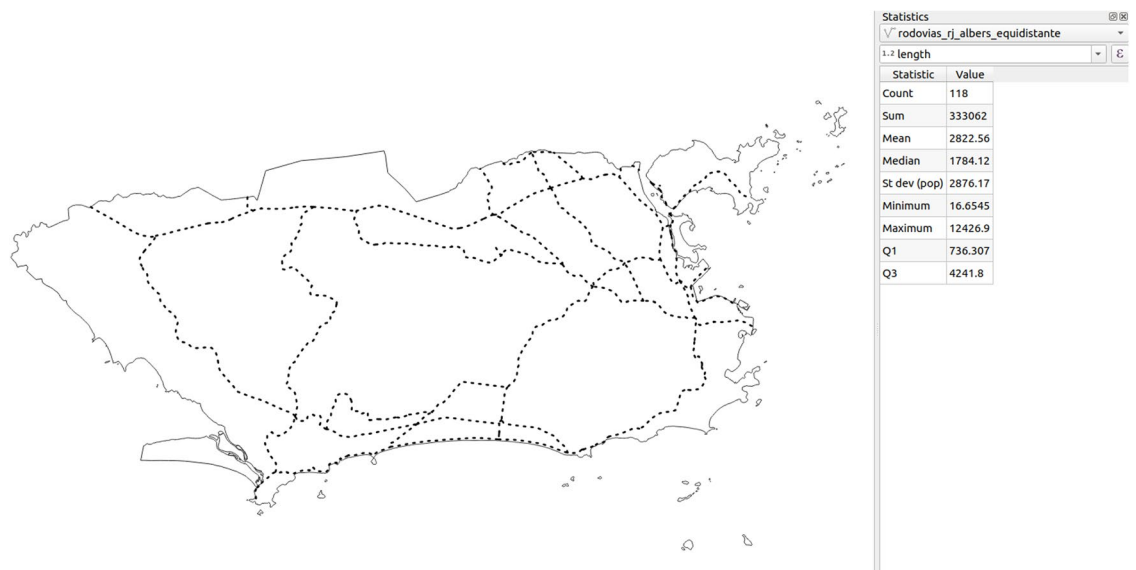
Fig. 6 Values of descriptive statistics calculated in QGIS for the Road class in the municipality of Rio de Janeiro (lengths in meters). The count statistic refers to the number of roads.
