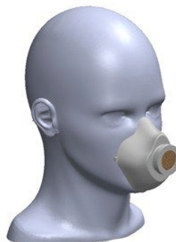
Fig. 2. Mask designed for a 3D scanned face for perfect fit and comfort.
