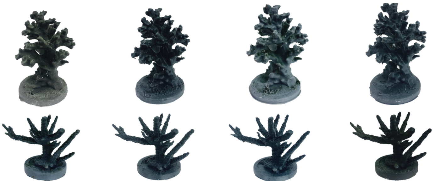
Fig 1. Replicates of P. damicornis (top) and A. formosa (bottom) control corals 3D printed with nGen, XT, PLA, and SS filament, respectively.
