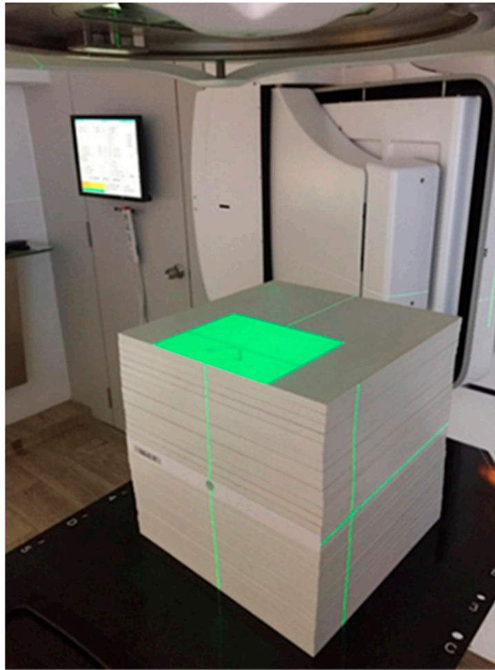
Figure 1. Picture of the 30 \times 30 \times 30 \text{ cm}^3 RW3 slab phantom incorporating the blood tube.
