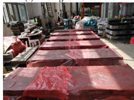
(e) Natural curing of UHPFRC
