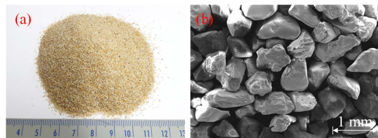
Figure 2. (a) Optical photograph and (b) microscale SEM image of Jumunjin sand.
