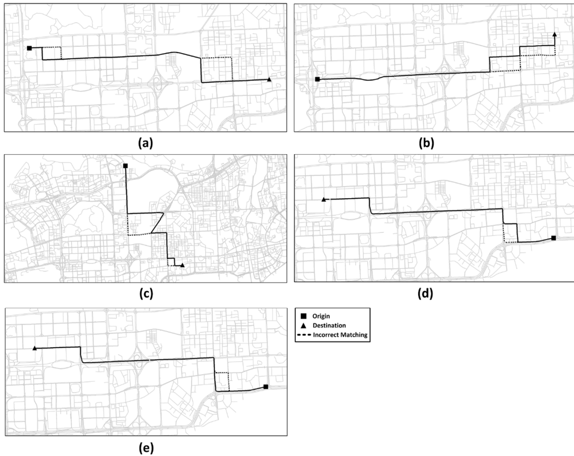
Figure 16. Incorrect map matching parts of ST-Matching algorithm. (a,b) Scenario T 1 . (c) Scenario T 2 . (d,e) Scenario T 3 .
