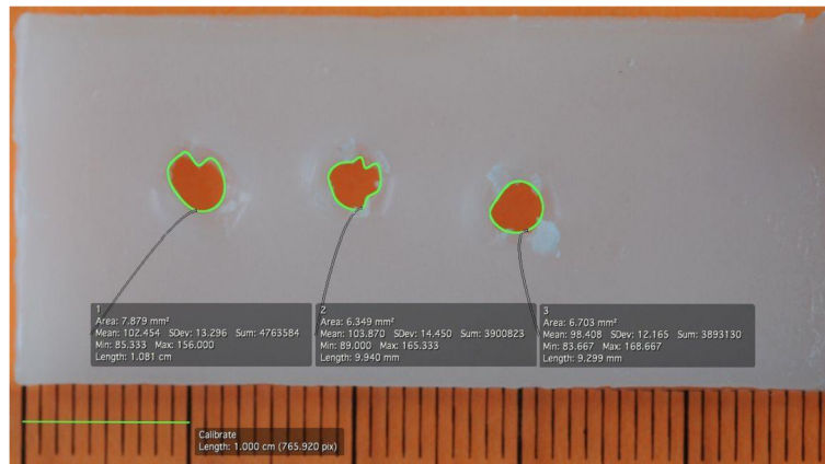
Fig. 3 Software to measure the area in mm 2 of the three perforation marks, which were set with each instruments. Twenty-one bonewax plates were used and sixty-three values could be obtained. Values were compared looking at instrument function and type
