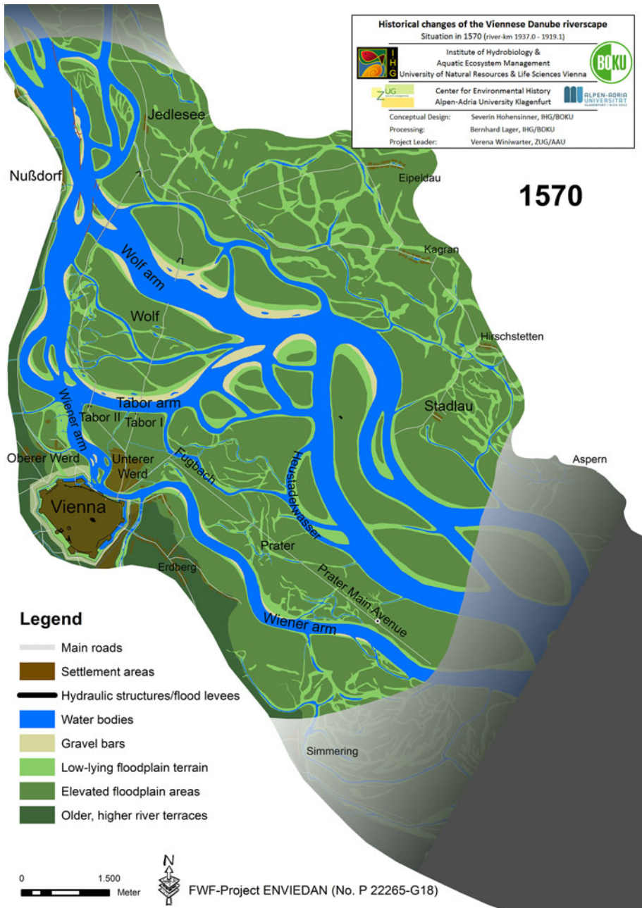
Fig. 2 Reconstructed state of the Danube riverscape in Vienna in 1570. The former main arm ( Tabor arm ) showed already significant sedimentation while the new main arm ( Wolf arm ) increased in width. Tabor I (until 1565) and Tabor II are indicated together with the bridges
