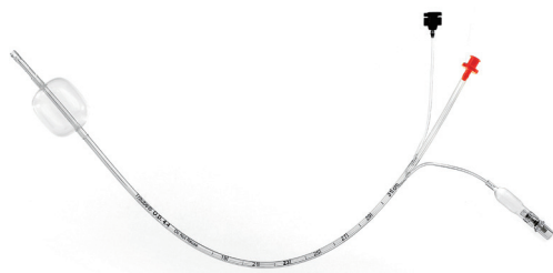
Figure 2 The Tritube is an endotracheal tube developed for flow controlled ventilation with one line for the cuff, a second line (red) for ventilation and a third line (black) for pressure measurements distal of the cuff. The tube has an inner diameter of 2.4 mm and an outer diameter of 4.4 mm (Ventinova Medical, Eindhoven, The Netherlands).
