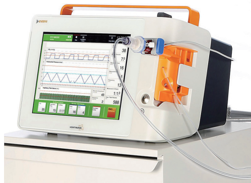
Figure 1 Flow controlled flow ventilation with the “Evone” ventilator. One main peculiarity of this technique is an active expiration according to the Venturi principle, controlled by pressure measurements distal of the cuff of the tube. This technique allows ventilation through a small catheter and leads to triangular in- and expiratory flow (lower curve on the monitor) (Ventinova Medical, Eindhoven, The Netherlands).
