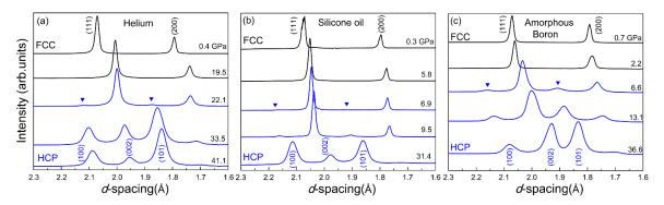
**Figure 3.** The in situ high-pressure XRD patterns of the CoCrFeMnNi HEA sample with helium (a), silicone oil (b), and amorphous boron (c) as the pressure mediums [53].
