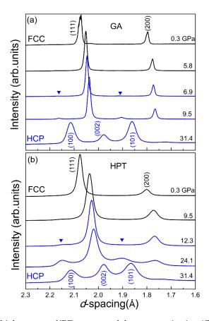
**Figure 4.** The in situ high-pressure XRD patterns of the gas-atomization (GA) and high-pressure torsion (HPT) CoCrFeMnNi HEA samples loaded in the same DAC with silicone oil as their pressure medium [53].
