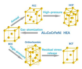
**Figure 7.** A schematic illustration of the atomic structure for five polymorphs observed in the  $Al_{0.6}$ CoCrFeNi HEA and the transition paths between them [62].
