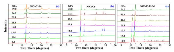
**Figure 5.** The XRD profiles of CoCrFeNi (a), CoCrNi (b), and CoCrFeNiPd (c) at high pressures: The diffraction peaks marked by symbol \* are from the Au pressure standard [57].
