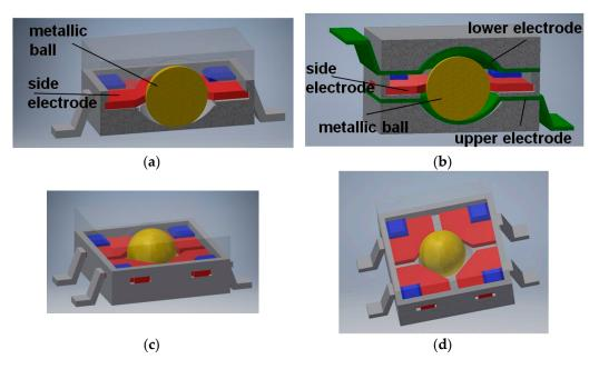
**Figure 4.** Dual-axis tilt switches: (**a**) with four electrodes; (**b**) with six electrodes; (**c**) arrangement of the side electrodes; (**d**) principle of operation.
