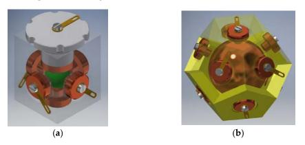
Figure 12. Tilt sensors based on the Platonic solids: (a) cuboidal sensor; (b) dodecahedral sensor.
