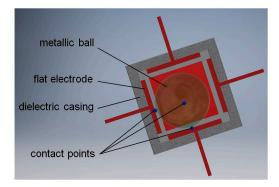
Figure 7. Principle of operation of a tilt sensor with eight detection sub-ranges.
