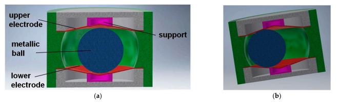
Figure 6. Dual-axis tilt switch with flexible electrodes: (a) the structure; (b) principle of operation.
