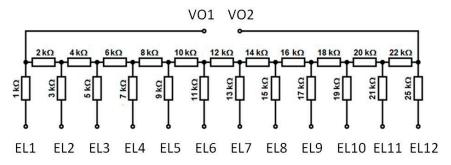
**Figure 16.** Resistance circuit created for the dodecahedron sensor illustrated in Figure 12b: EL1–EL12, electrodes of the sensor; VO1–VO2, analog voltage outputs.
