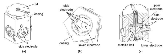
**Figure 10.** Tilt sensor in a form of pentagonal prism: (**a**) perspective view; (**b**) inside chamber; (**c**) establishing of electric contact (short-circuiting of the lower and the two side electrodes).
