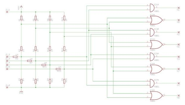
**Figure 15.** Logic circuit for the sensor in the form of the cuboidal sensor presented in Figure 12a: EL1–EL6, electrodes of the sensor; Y1–Y8, digital outputs corresponding to particular vertices.
