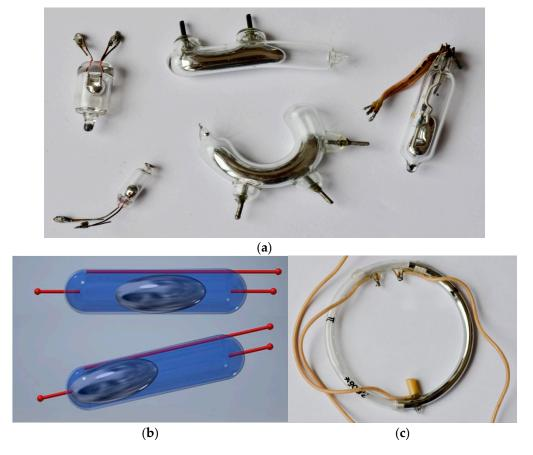
Figure 1. Mercury tilt sensors: (a) various types of contact switches; (b) principle of operation; (c) sensor with resistive wire.
