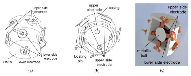
**Figure 13.** Dodecahedral tilt sensor: (**a**) perspective view; (**b**) inside chamber; (**c**) establishing of electric contact (short-circuiting of the upper side and two lower side electrodes).
