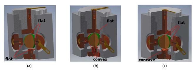
Figure 14. Possible shapes of the contact surface of the lower electrode: (a) flat; (b) flat and convex; (c) flat and concave.
