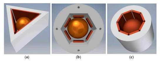
**Figure 9.** Tilt sensors with prismatic shape and spherical free element (view without the upper electrode): (**a**) triangular prism; (**b**) hexagonal prism; (**c**) octagonal prism.
