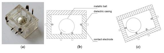
Figure 2. Single-axis tilt switch: (a) photograph; (b) general diagram; (c) principle of operation.
