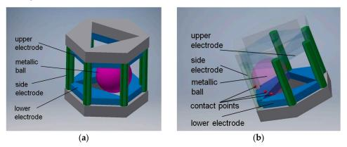
Figure 8. Sensor with six detection sub-ranges: (a) the structure; (b) principle of operation.
