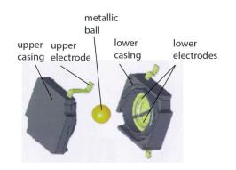
Figure 3. Dual-axis tilt switch by Alps Electric.
