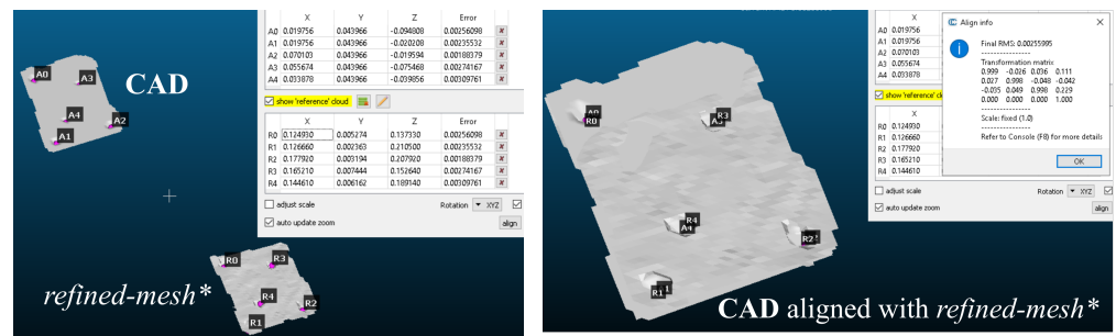
Figure 19. To perform a comparison between meshes, they need to be first aligned to each other. This was done by point set registration (in CloudCompare ) with control points defined as the the clusters obtained from Gaussian curvature evaluation over both the CAD and refined-mesh* .
