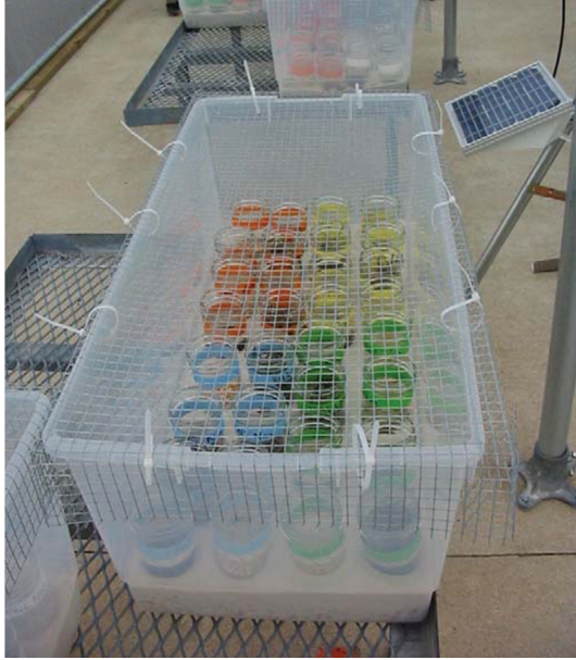
FIGURE 2: Photograph of samples of M. bovis inoculated substrates in their primary containers placed within their secondary containers inside the experimental environmental sample enclosure. Shown here are the “nonshaded” treatments from 4 sample sets (total of 32 sample jars).
