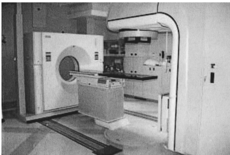
FIG. 1. (Color) CT scanner in the same room as a linear accelerator, sharing a single patient couch.
