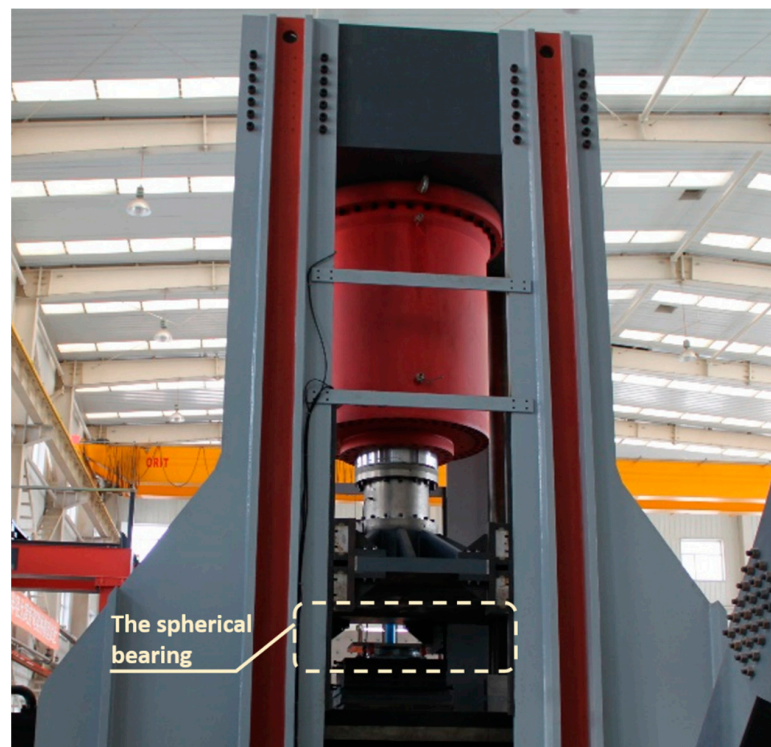
Figure 7. YAJ-30000 KN microcomputer controlled electro-hydraulic servo press shear test machine.
