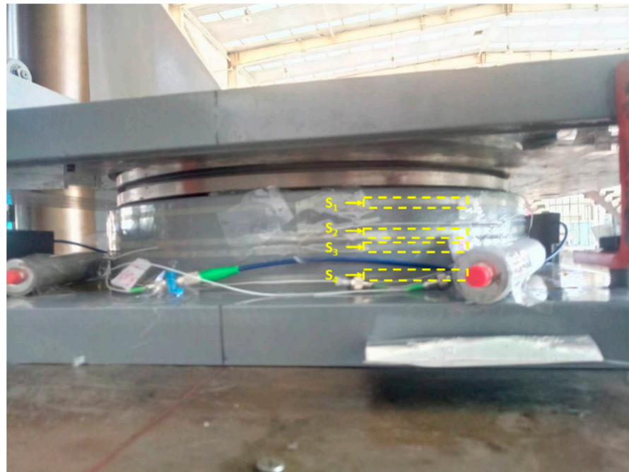
Figure 4. The picture view of load-sensitizing spherical bearing. S_1 , S_2 , S_3 : the three sensing fibers located at the upper region of the pot support; S_4 : the reference fiber, acting as a temperature compensation fiber.
