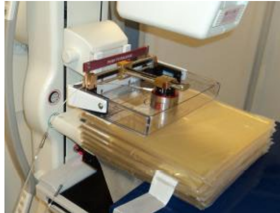
FIG. 4. Setup for the skin-to-center dose measurements using OSLDs and a phantom comprised of flexible tissue-equivalent bolus material. For each measurement, two OSLDs were placed along the central axis of the two applicators, one at the phantom midplane and the other at the phantom surface.
