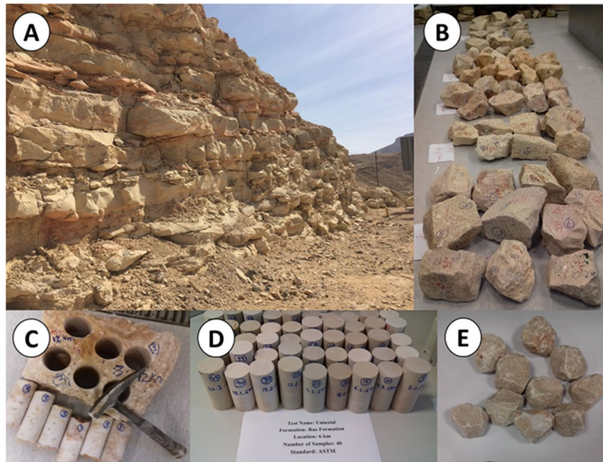
Figure 2. (A) General view of the Rus Formation and limestone outcrops, (B) a group of rock blocks collected from the field and used for coring and testing, (C) a cored rock block sample with core samples, (D) core samples prepared for the UCS test, and (E) test sample for the SDI test.
