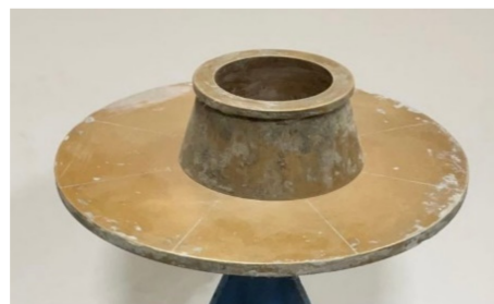
Figure 3. Mortar flow test apparatus.
