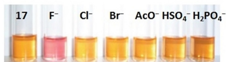
Figure 12. TTF-functionalized DPQ, 17 for selective fluoride sensing. Fluoride selective color changes observed for 17 in \text{CH}_2\text{Cl}_2 . Reprinted from Ref. [39] with permission. Copyright (2012) Royal Society of Chemistry.
