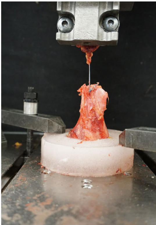
Figure 7. A right shoulder from the biceps button group during cyclic loading, showing large displacement after slipping and tearing of the suture through the tendon.
