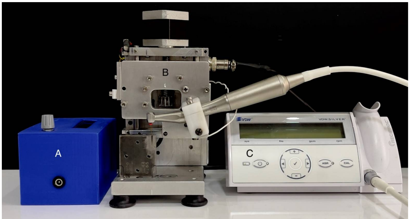
Figure 1. Dynamic cyclic fatigue test setting: (A) control panel, (B) dynamic device and artificial canal, and (C) VDW Reciproc Silver.
