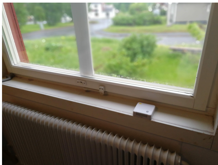
Figure 5. Sensor E8 beside a 2 layer glass window inside of a wooden house.
