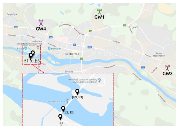
Figure 3. S1—gateways and sensors positioning. Map layer from Google Maps [41].
