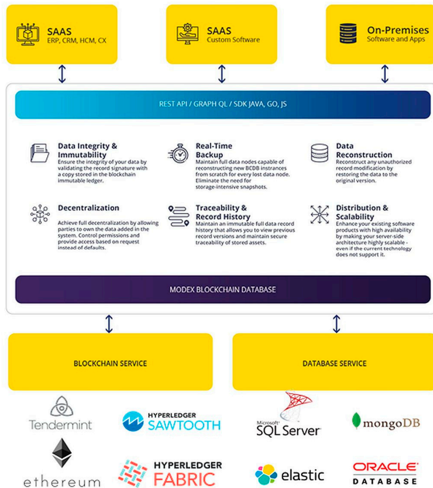
Figure 3. Modex Blockchain Database (BCDB) infrastructure [62]. Reproduced with permission from Modex Ltd.; published on the www.modex.tech website, 2020.
