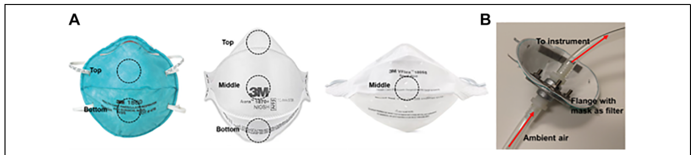
Figure 2. Forced particle penetration of N95 FFRs. Three types of 3M N95 FFRs were used in this study: model 1860, model 1805, and model 1870/1870+. (A) Regions of each FFR tested for particle penetration. (B) An example of a model 1860 mounted and connected to an Aerotek Portable Particle Counter. A total of 283 L of air was forced through each 1-inch-diameter test section of the mask.
