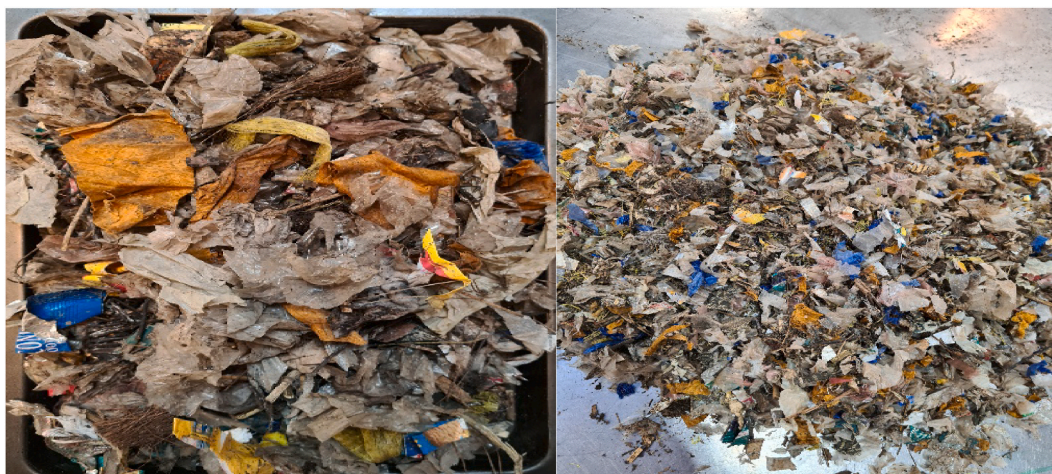
Fig. 4. MSW Feedstock before (left side) and after (right side) crushing for slurry.
