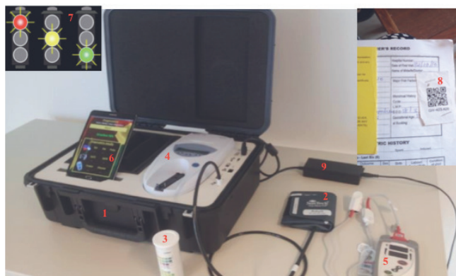
Figure 1. B4M device. 1 – Portable water and heat resistant dustproof case; 2 – Automated blood pressure cuff; 3 – Urinary glucose and protein Chemistrips; 4 – Urisys 1100® Urine Analyzer; 5 – Pronto-7® Rainbow Pulse CO-Oximetry device; 6 – Android tablet with decision support algorithms; 7 – Traffic-signaling alert system; 8 – Unique QR code for easy tracking and recall of patient records; 9 – AC adapter for charging the device.
