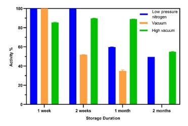
**Figure 7.** Shelf-life test of the TEMPO-CNC glucose sensor under different storage conditions: low-pressure nitrogen (400 mbar  $N_2$ ), vacuum (≤50 mbar), and high-vacuum (≤10 mbar) drying treatment before vacuum packing (≤50 mbar). All sensors were stored at 4 °C. The sensors were tested after 1 week, 2 weeks, 1 month, and 2 months. All values are normalized against the signals of sensors tested without storage.
