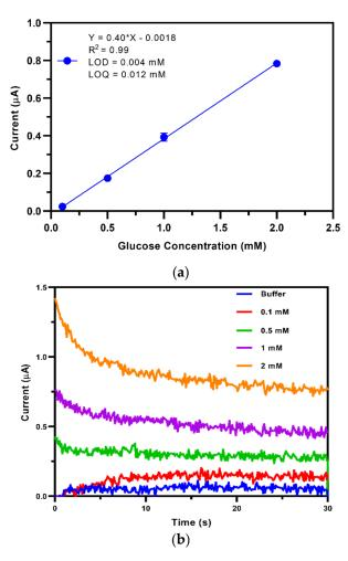
**Figure 4.** (a) Raw data sets of chronoamperometry measurements with the TEMPO-CNC glucose sensor in phosphate buffer containing 0.1–2 mM glucose. (b) Calibration curve of the TEMPO-CNC glucose sensor in 0.1–2 mM glucose in phosphate buffer. The linear range (up to 2 mM) was smaller than the entire dynamic range. n = 3; plotted are the mean  $\pm$  standard deviation and the linear fit from 0.1 to 2 mM.
