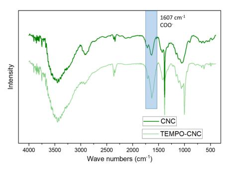
**Figure 2.** FTIR spectra of cellulose nanocrystals (CNCs) (dark green curve), TEMPO CNCs (light green curve curve).
