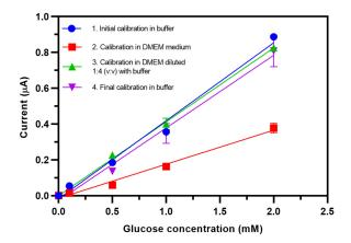
**Figure 8.** Calibration curve of a single TEMPO-CNC glucose sensor in the range from 0.1 to 2.0 mM glucose in the following order: (1) Phosphate buffer, (2) DMEM medium, (3) diluted DMEM medium (1:4 [v:v] with phosphate buffer), and (4) phosphate buffer. DMEM refers to DMEM medium supplemented with 10 % serum and 1 % antibiotics. All data points represent mean values  $\pm$  standard deviation of three measurements.
