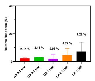
**Figure 5.** Relative responses of the TEMPO-CNC glucose sensor toward interfering species (0.1 mM L-ascorbic acid, 0.1 and 1 mM uric acid, 0.1 and 1 mM L-lactic acid) in a 1 mM glucose standard solution in phosphate buffer. n = 3 for each condition; 1 mM glucose without interfering species is defined as 100 % response.
