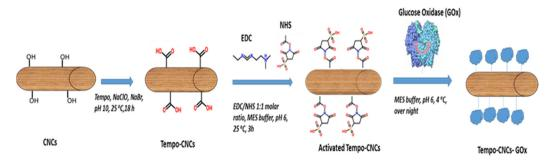
Figure 1. Schematic view of the TEMPO-CNCs oxidation and enzyme immobilization process.
