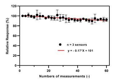
**Figure 6.** Operational stability of the TEMPO-CNC glucose sensors over 30 repeated measurements in 1 mM glucose solution in phosphate buffer. The graph depicts the average values of three individual sensors (mean  $\pm$  standard deviation); the red linear fit indicates the loss in measured current over the 30 cycles (total of 6 h of measurement). The average remaining activity of the TEMPO-CNC glucose sensor after 30 measurements was 92.3% of the initial current.
