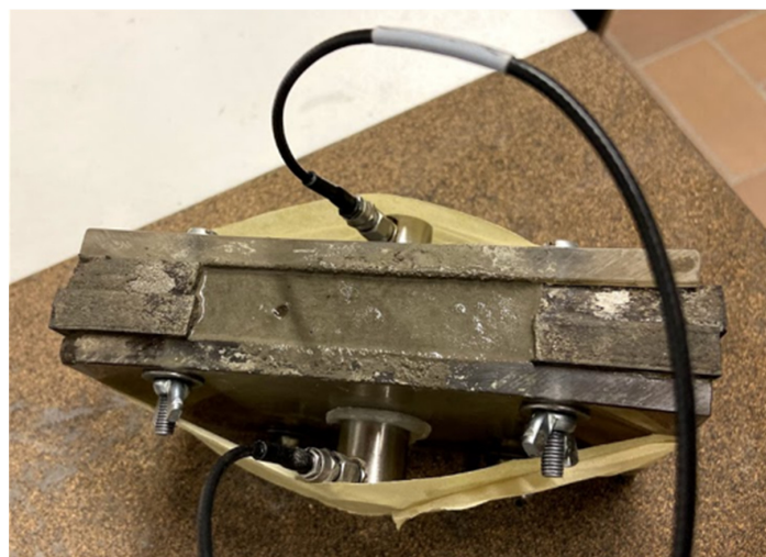
Figure 2. Ultrasound set-up showing the mortar sample in between both sensors.
