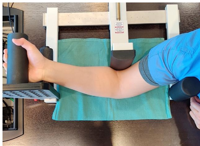
**Figure 1** Telos positioning. Subject seated upright with arm in 15–30° of flexion in a Telos SD900 stress machine with a fixed 5N of valgus stress applied across the elbow.
