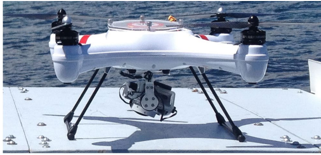
Figure 1. Splashdrone (SwellPro, Shenzhen, China) on custom built foldable helipad on research vessel, AUT Sciences .
