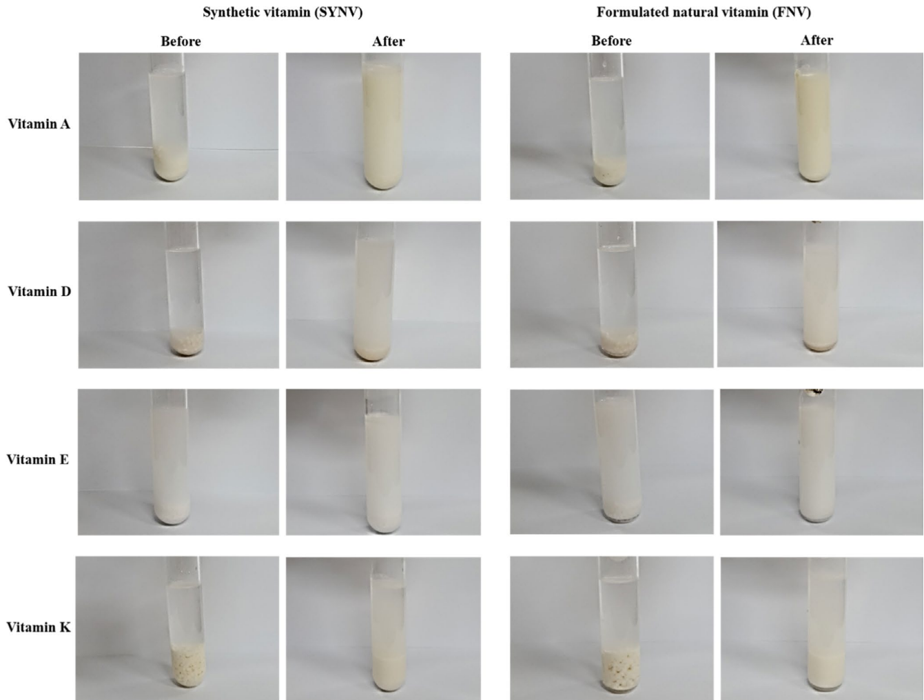
FIGURE 3 Dispersion test-left: before and after dispersing SYNV; right: before and after dispersing FNV A, D, E, and K in the water at 37°C for 30 min
