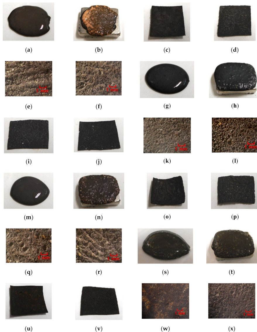
Figure 7. Images of liquid before electrolytic polymerization and mixing electrolytically polymerized rubber with water-insoluble MF: (a–f) MSGS60; (g–l) A500; (m–r) HC50; (s–x) DS50; (a,g,m,s) liquid before electrolytic polymerization without magnetic field; (b,h,n,t) liquid before electrolytic polymerization under magnetic field; (c,i,o,u) panoramic image of electrolytically polymerized rubber facing anode; (d,j,p,v) panoramic image of electrolytically polymerized rubber facing cathode; (e,k,q,w) microscopic image of electrolytically polymerized rubber facing anode by optical microscope; (f,l,r,x) microscopic image of electrolytically polymerized rubber facing cathode by optical microscope.
