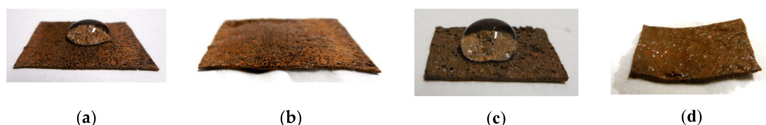
Figure 16. Images of MCF rubber before and after water permeation: (a) before permeation (0.75 g MF, 0.5 g \text{TiO}_2 , 3 g S-500, 3 g 671A, and 3 g Ni); (b) after permeation (0.75 g MF, 0.5 g \text{TiO}_2 , 3 g S-500, 3 g 671A, and 3 g Ni); (c) before permeation (3 g KF96, 3 g PVA, 0.75 g MF, 0.5 g \text{TiO}_2 , 3 g S-500, 3 g 671A, and 3 g Ni); (d) after permeation (3 g KF96, 3 g PVA, 0.75 g MF, 0.5 g \text{TiO}_2 , 3 g S-500, 3 g 671A, and 3 g Ni).
