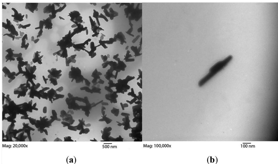
**Figure 5.** SWCNT subjected to 4 h 7 mol/L nitric acid reflux prior to functionalization and dialysis, resulting in stubbier tube bundles. (a) 20,000 $\times$ ; (b) 100,000 $\times$ .
