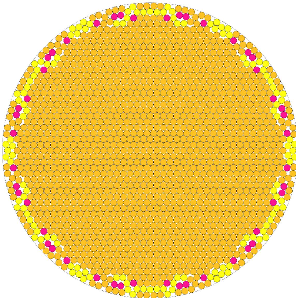
**Figure 6.** Code output derived cartoon showing optimal packing of 1735 circles of equal radius in a larger circle. Yellow and pink colored circles correspond to predicted loosely packing nanotubes in the outermost layers of the bundle as bundling energy is decreased with available surface area.
