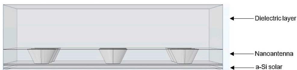
Figure 11. Side view of the 3D a-Si solar cell structure with nanoantenna with conical holes.
