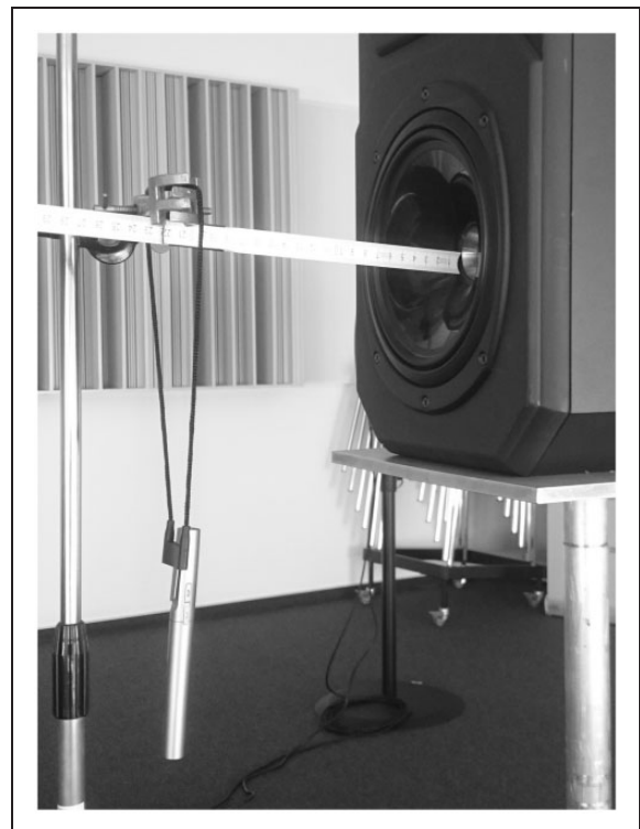
Figure 3. Position of the RM in front of the coaxial chassis of the far field speaker. The folding yardstick is used to show the spacing between far field speaker and RM—it is removed during the tests.
