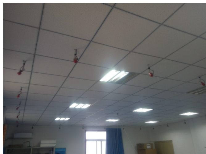
Figure 4. OptiTrack motion capture system.
