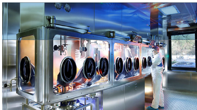
Figure 7. Glove box environment at Bayer's Wuppertal development site to manufacture highly potent active ingredients.
