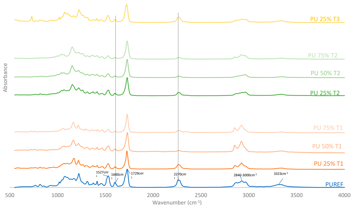
Figure 2. FTIR spectra of the HMPUR adhesives based on different biobased polyols (T1, T2 and T3, respectively), and different content of biobased polyols.
