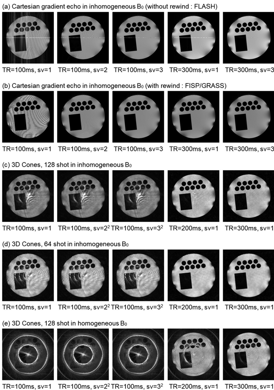
Fig. 5 Simulated images calculated for Cartesian sampling gradient-echo and 3D Cones sequences for various TRs and numbers of subvoxels. (a) The Cartesian gradient-echo sequence in an inhomogeneous magnetic field without rewinding phase-encoding gradients. (b) The Cartesian gradient-echo sequence in an inhomogeneous magnetic field with rewinding phase-encoding gradients. (c) 128-shot and 256-cone 3D Cones sequence in an inhomogeneous magnetic field. (d) 64-shot and 256-cone 3D Cones sequence in an inhomogeneous magnetic field. (e) 128-shot and 256-cone 3D Cones sequence in a homogeneous magnetic field. FLASH, fast low angle shot; FISP, fast imaging with steady-state precession.
