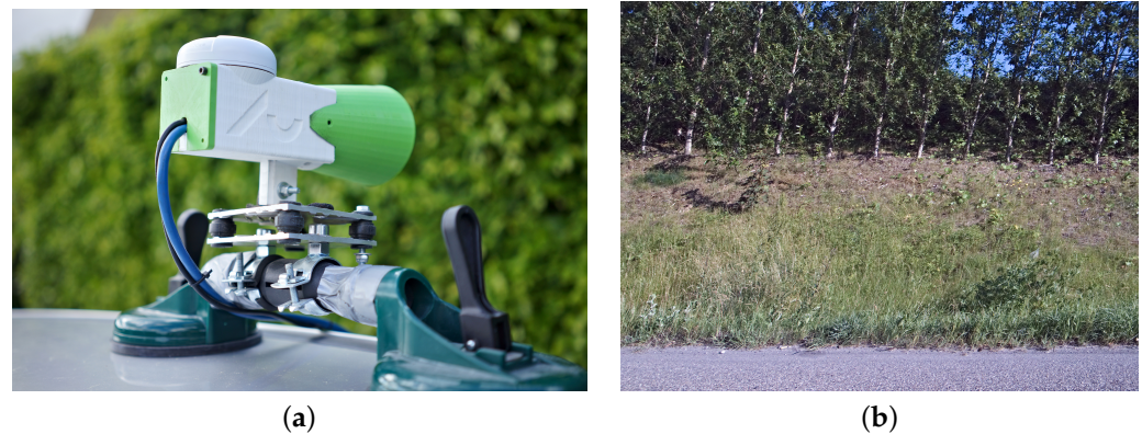
Figure 4. (a) The selected camera system that is tested at speeds up to 130 km/h. It consists of Daheng MER-1220-32U3C camera with 8mm lens and u-blox 8 UBX-M8030-KT GNSS receiver that are mounted on the car roof with suction cups. (b) Sample from Daheng MER-1220-32U3C with an 8 mm lens and 100 \mu s exposure time, while driving 110 km/h. Notice the leaning of the trees, which is a result of the rolling shutter.
