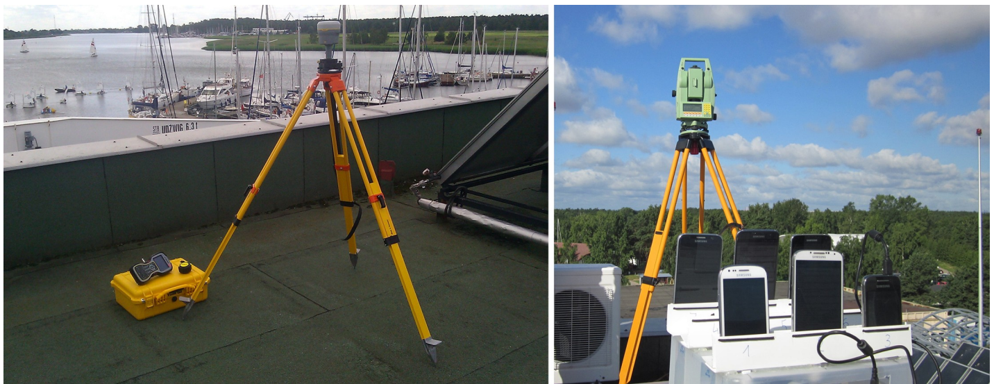
Fig 3. Establishment of the control network points using static satellite measurements (left) and determination of the position coordinates of the measurement station by the tachymetric method (right).
