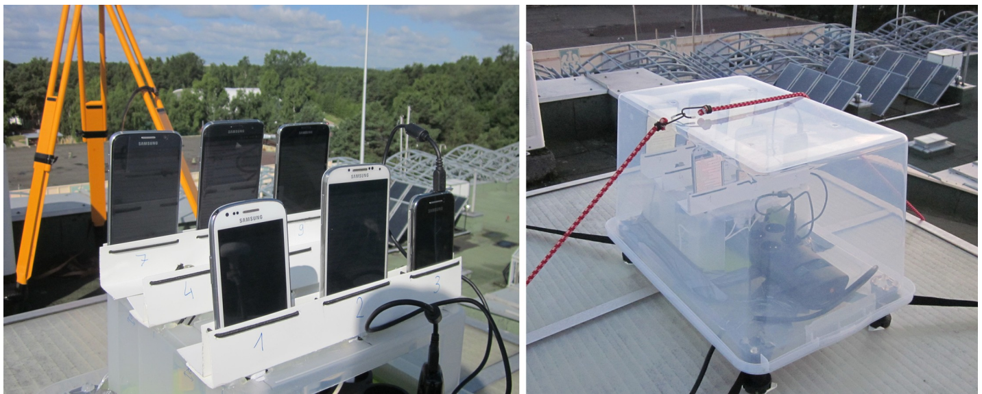
Fig 2. Measurement platform with attached mobile phones (left) and a plastic cover mounted (right).
