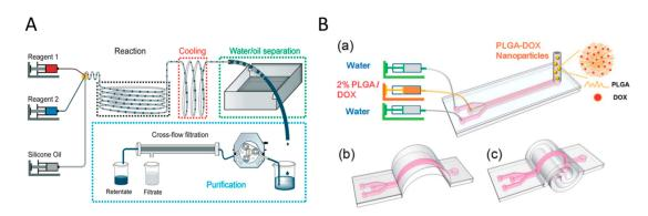
**Figure 5.** Schematic of modular microfluidic systems for producing NPs. (**A**) A droplet-reactor system with the potential for automation. Reprinted with permission from ref [105]. (**B**) A microfluidic origami chip with different configurations for enhancing mixing. Reprinted with permission from ref [106].
