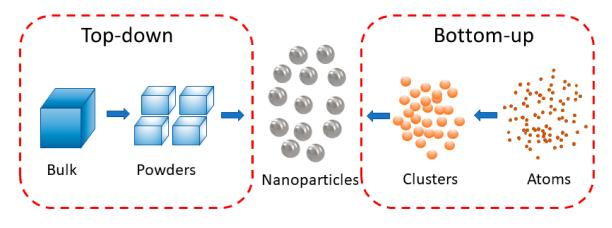
Figure 1. Scheme of top-down and bottom-up synthesis of nanoparticles (NPs).
