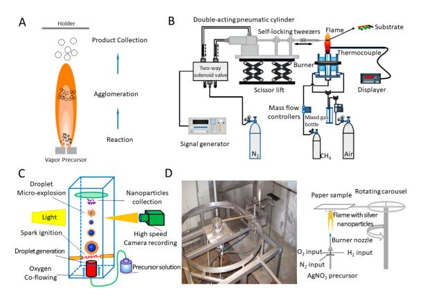
**Figure 6.** Flame synthesis systems for producing NPs. (**A**) Schematic representation of a typical flame synthesis system. (**B**) Schematic of methane coaxial jet diffusion flam system. Reprinted with permission from ref [111]. (**C**) Experimental setup for single isolated droplet combustion. Reprinted with permission from ref [112]. (**D**) The setup and schematic of the liquid flame spray (LFS) system. Reprinted with permission from ref [92].
