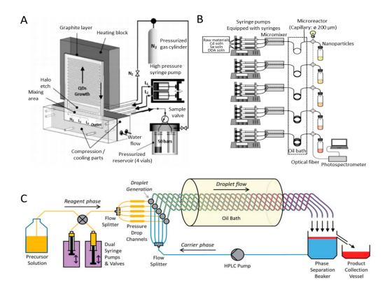
**Figure 4.** Microfluidic/millifluidic systems for producing NPs. (**A**) microfluidic system for producing CdSe quantum dots (QDs). Reprinted with permission from ref [94]. (**B**) A combinatorial synthesis system contains several microreactors for CdSe NPs production [95]. (**C**) A multichannel droplet microfluidic reactor. Reprinted with permission from ref [91].
