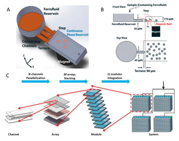
**Figure 7.** Microfluidic systems for producing microparticles (MPs). (**A**) Schematic view of a magnetically driven microfluidic droplet generation technique using ferrofluids (without any pumps). (**B**) Top and front views of the microfluidic device with dimensions. Reprinted with permission from ref [130]. (**C**) Overview of multidimensional scale-up strategy (not to scale). Reprinted with permission from ref [134].
