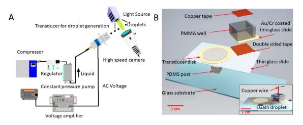
**Figure 9.** Schematics of acoustic systems for MPs production. (**A**) Schematic of a droplet generation system incorporating an ultrasonic torsional transducer and a micropore plate. Reprinted with permission from ref [150]. (**B**) Exploded schematic of the acoustic-based LM microdroplet production platform. The inset is the assembled view. Reprinted with permission from ref [48].
